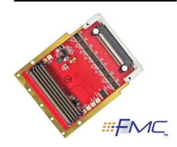
The NES-FMC34DF is a VITA57 FPGA Mezzanine module. The front bezel has a Samtec ERF8-040-01-L-D-RA-L-TR connector. We use 6 Samtec RSP-122811-01 connectors as three differential pairs for transferring signals to the HB bank. These are useful for providing external-clock/ synchronization-signals.
